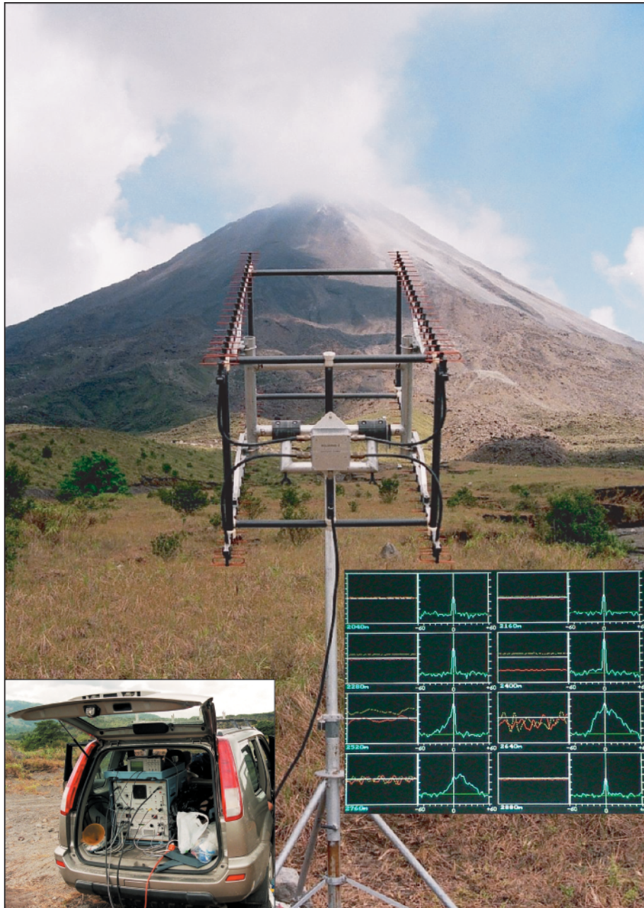
Fig. 1. The VOLDORAD (Volcano Doppler radar) antenna aimed at the summit of Arenal volcano 2.5 km away; the operating radar is in a four-wheel-drive vehicle (left inset) and provides signal real-time screen monitoring during an explosion (right inset).
