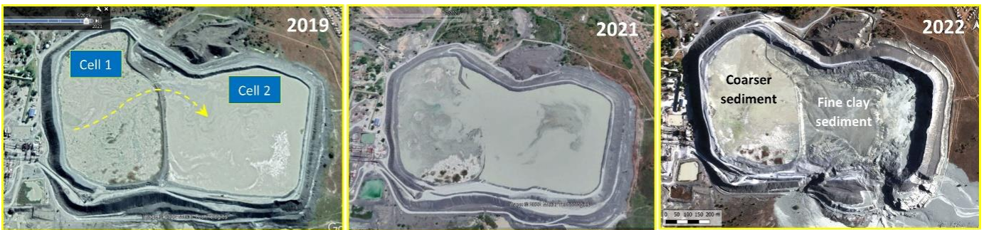
Figure 4: Time sequence for the Jagersfontein TSF failure.
