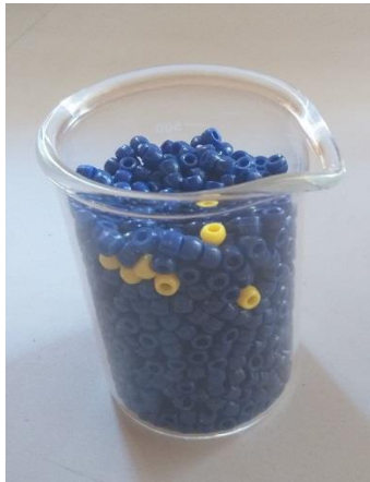
Figure 2. A flask containing inhomogeneously distributed yellow beads in a ratio of 5000 g/tonne, or 5000 ppm.
