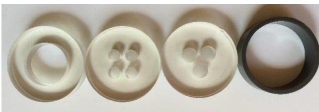
Figure 2: some examples of the acrylic disks commonly used by the Potsdam SIMS lab.
